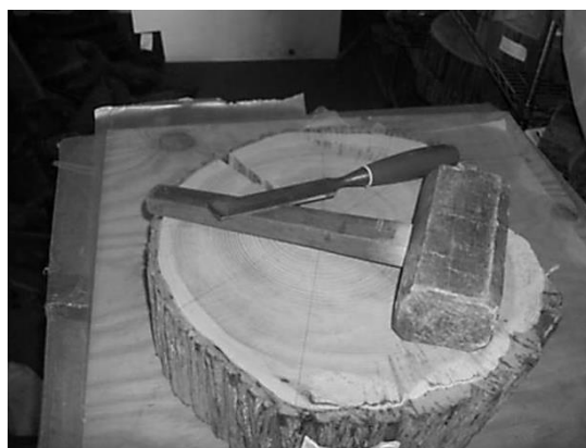
Figure 4. Chisel and hammer tools from Colonial Williamsburg Master Craftsman, Name, used to collect 10-year increments of selected bolewood cookies. De-ionized water rinses and food grade wax paper barriers were used to ensure clean surfaces.
